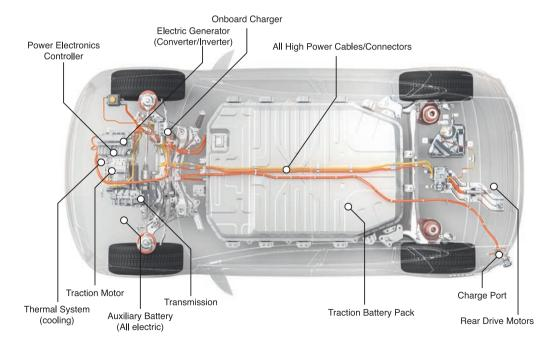
**Battery (all-electric auxiliary):** In an electric-drive vehicle, the auxiliary battery provides electricity to power the vehicle's accessories.
